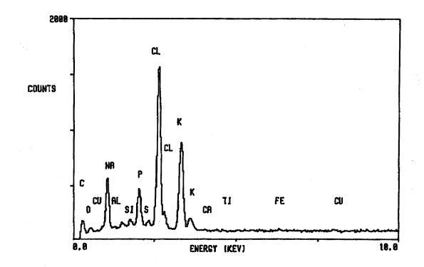
Fig. 11 - SEM/EDX spectrum of the blue gel-like substance
