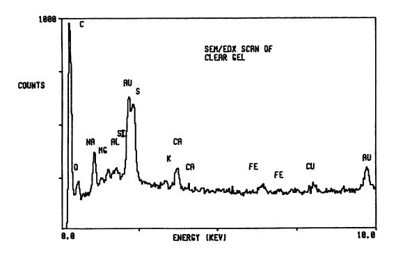
Appendix 3 – Fig. 13 – SEM/EDX scan of embalming gel, sample # 3
