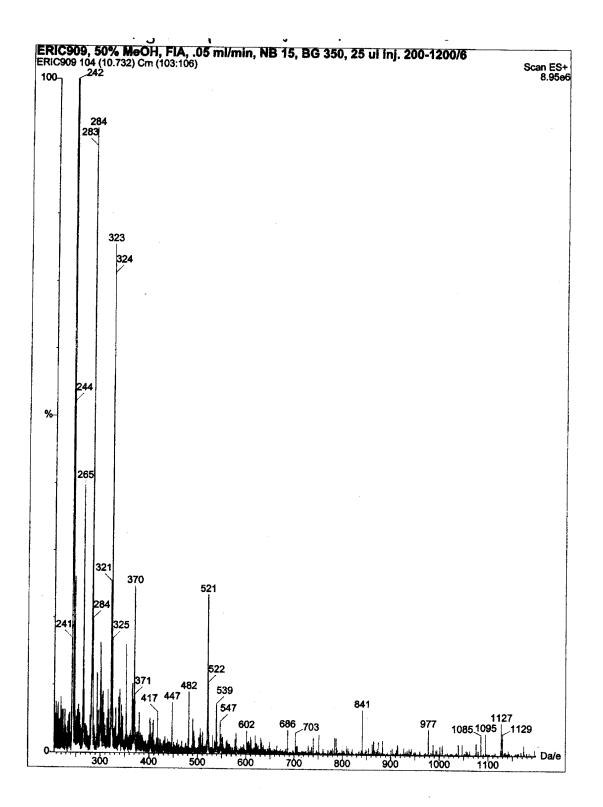
Fig. 14 – Spectrum of blue gel-like substance
