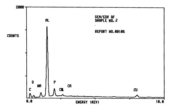
Appendix 3 – Fig 1 – SEM/EDX scan of embalming gel # 1
