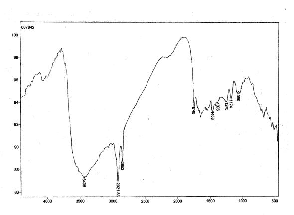
Fig. 12 – Infrared spectrum of the blue gel-like substance.
