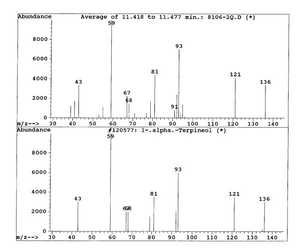
Appendix 3 – Fig. 9 – Compound E from TIC of embalming gel # 2 identified as 1- alpha-terpineol
