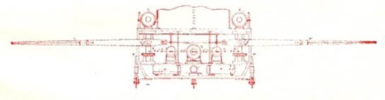
LEGEND: G. Steam Boiler H. Engine J. Oil Tank K. Air Vessel L. Air Heater P. Pivot T. Turning Wheel W. Wing
