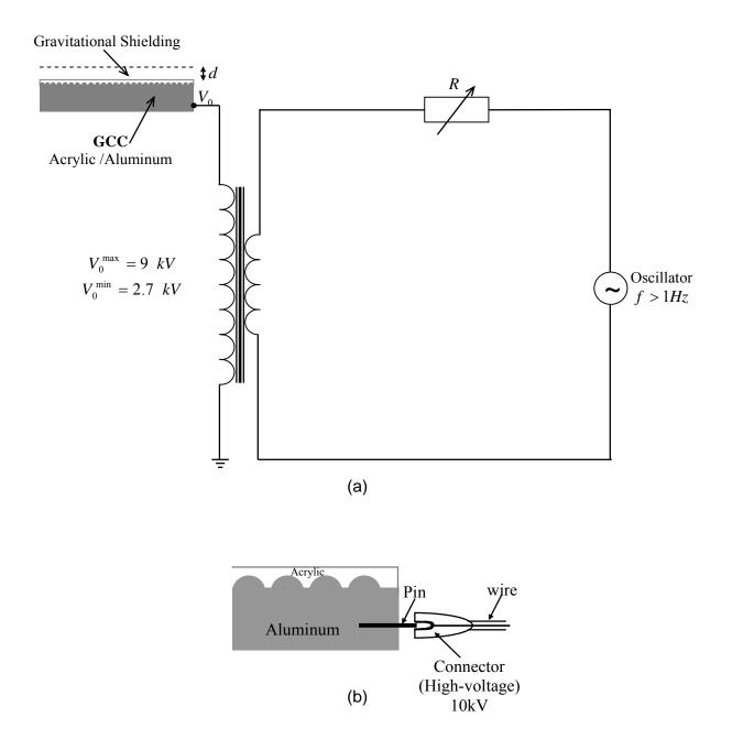
Fig. A10 – (a) Equivalent Electric Circuit. (b) Details of the electrical connection with the Aluminum plate. Note that others connection modes (by the top of the device) can produce destructible interference on the electric lines of the  $E_{\rm air}$  field.
