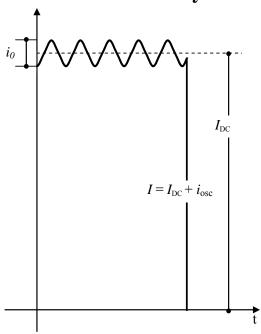
Fig. A1 - The electric current I varies with frequency f. But the variation of I is quite small in comparison with  $I_{DC}$  due to  $i_o << I_{DC}$ . In this way, we can consider  $I \cong I_{DC}$ .
