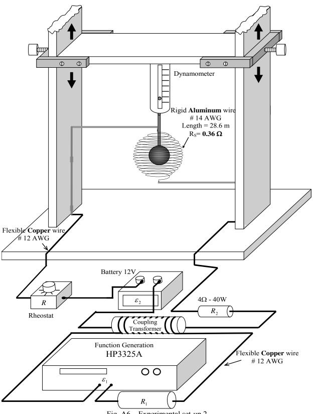
Fig. A6 – Experimental set-up 2.
