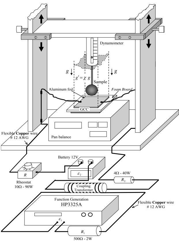
Fig. A2 – Experimental Set-up 1.
