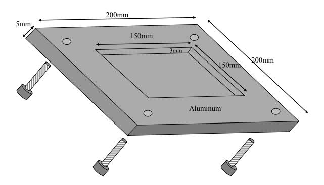
Fig.B1 – Mold design
